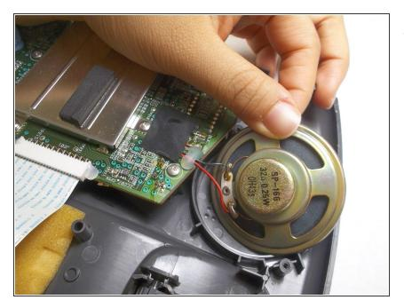
Solder your replacement speaker into the circuit. For assistance with soldering check out the <u>iFixit Solder</u> and Desolder Guide.
