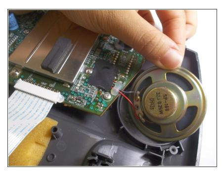
• Finish speaker removal by cutting both the black and red wires.
