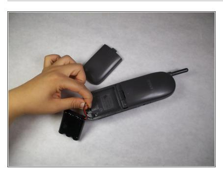
Remove the rechargeable battery pack (BP-T18) by pressing down on the power cable connector and pulling at the same time. To reassemble your device, follow these instructions in reverse order.
