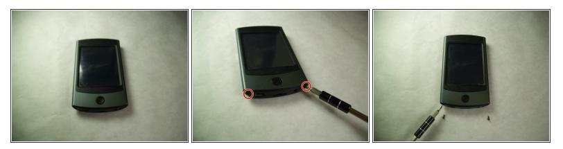
Using the screwdriver with the J00 bit, remove the two 4.8 mm Phillips screws.
