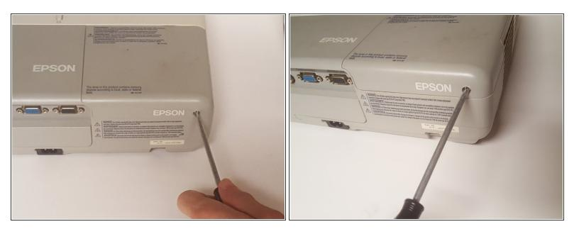
• Using a Phillip's head screwdriver, remove the screw from the back.
