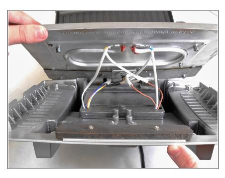
Slightly lift the silver plate from the grill base to reveal the interior wiring
