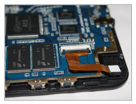
Near the top left of the device, gently unclip the gold ribbon cable by pulling up the black clip holding it in place and removing the ribbon.
