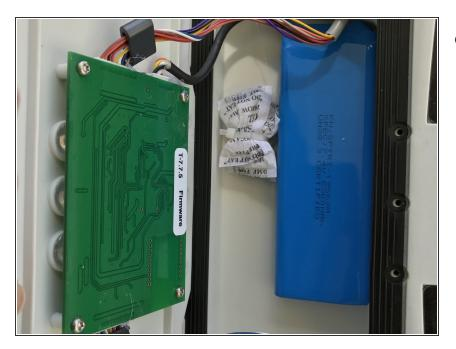
Battery pack, desiccant and bottom of board showing T-7.7.5 firmware revision number label.
