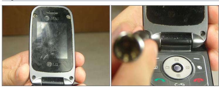
Remove the four 3mm #000 flat Phillips head screws from the front screen using a Phillips #000 Screwdriver.
