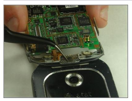
Use tweezers to remove the top ribbon cable, mentioned in step 11, from the hinge area.
