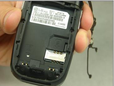
• Remove the sim card by sliding the card out from under the retainer using either your fingers or a spudger.
