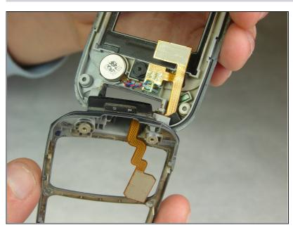
You can now carefully pull apart the phone casing at the hinge by separating them at the left side of the hinge.
