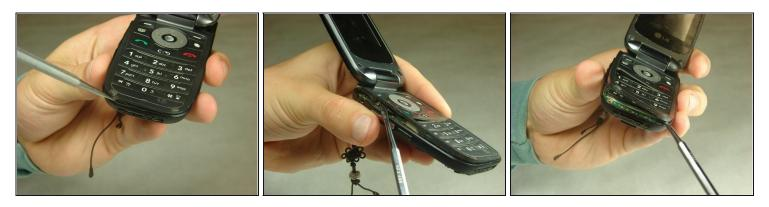
Insert the metal spudger between the keypad assembly and back cover assembly and pry the two assemblies apart.
