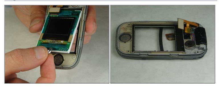
• Grip the screen and ear speaker connected to the screen via red and black wires, and carefully pull the screen away from the screen assembly.
