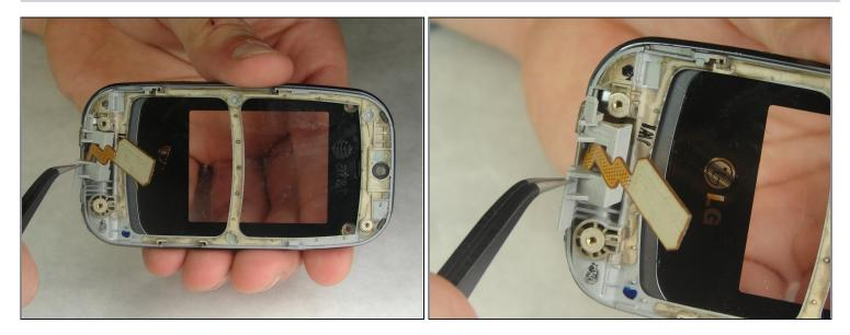
• Using <u>tweezers</u>, pull the gray plastic piece that is going around the flex cable out of the hinge area.
