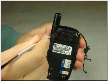
• Remove the rubber covers in the highlighted locations using a metal spudger.
