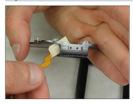
• Carefully slide the display flex cable out.
