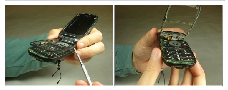
Once you have worked your way around the perimeter of the phone, you will have access to the components in the bottom half assembly.
