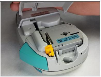
Push on the side of the cover, and pull up to remove it.
