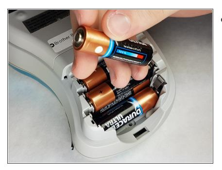
• Remove the batteries.
