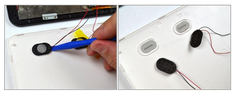
Remove the old speakers from the back cover with the plastic prying tool.
