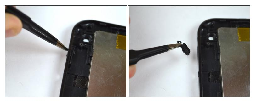
• Push the power button towards the interior of the device to free it from its slot, using tweezers.
