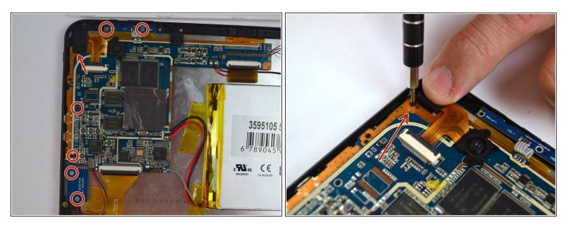
Remove all of the 4mm screws that attach the motherboard to the rest of the device.
