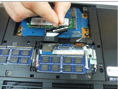
Using the pull tab, disconnect the black solid-state drive cable from the system board.
