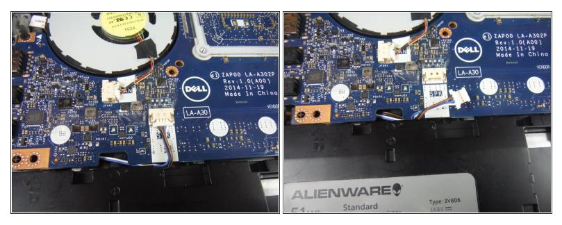
• Disconnect the speaker cable connector from the service board.
