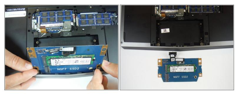
• Lift up on the solid-state drive assembly to remove it from the computer base.
