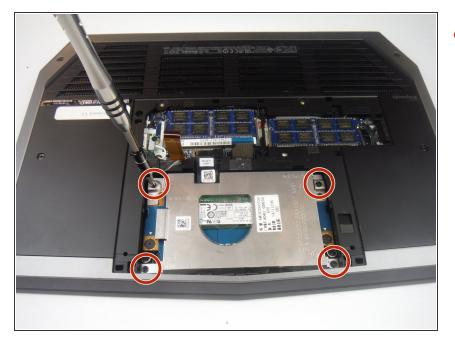
Remove (4) 6 mm Phillips head screws from the solid-state metal drive bracket, using a Phillips # 1 screwdriver.
