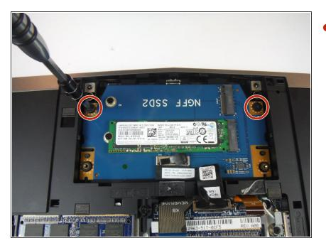
Remove (2) 3 mm Phillips head screws, using a Phillips # 0 screwdriver, that connect the solidstate drive assembly to the computer base.
