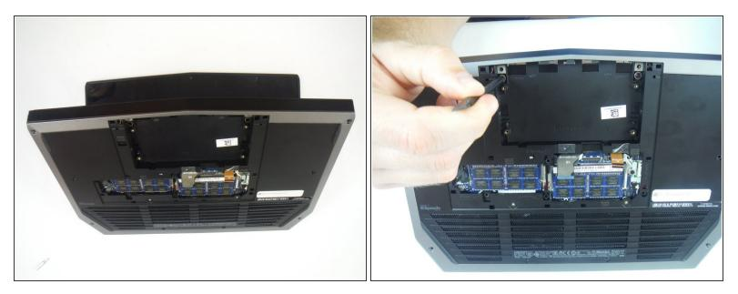
Lift the computer base slightly towards you and push the release tabs on the palm-rest assembly until it pops out using a spudger.
