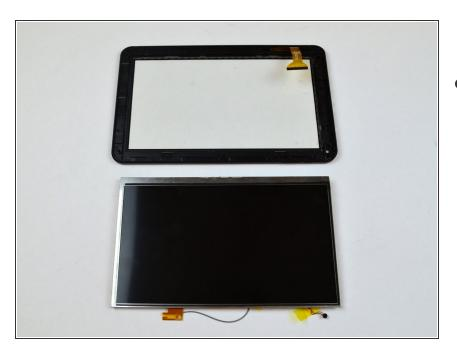
Completely remove the display screen from the touchscreen. To reassemble your device, follow these instructions in reverse order.
