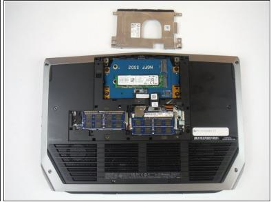
Grab the pull tab to pivot the solid-state drive bracket upwards. Remove the bracket from the computer base.
