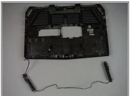
After removing the battery, lift up on the speakers and wires to fully removed from the base panel.
