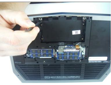
• Lift the computer base slightly towards you and push the release tabs on the palm-rest assembly until it pops out using a spudger.
