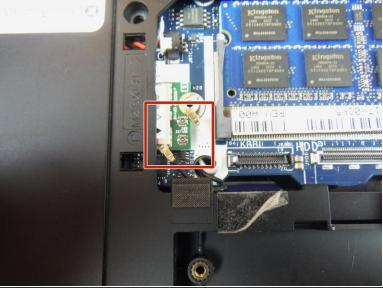
Disconnect the antenna cables from the wireless card using a heavy duty spudger. The wires can be removed by applying a force directed upward, away from the device.
