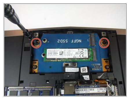
Remove (2) 3 mm Phillips head screws, using a Phillips # 0 screwdriver, that connect the solidstate drive assembly to the computer base.
