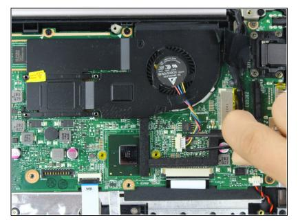
• Disconnect the fan's power cable by pulling upward on the pin connector with a pair of <u>tweezers</u>.
