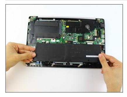
• Lift and remove the battery.
