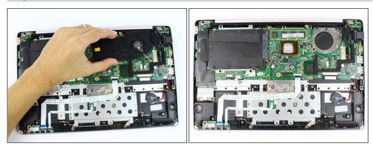
• Grab the sides of the fan assembly and remove it by lifting upwards.
