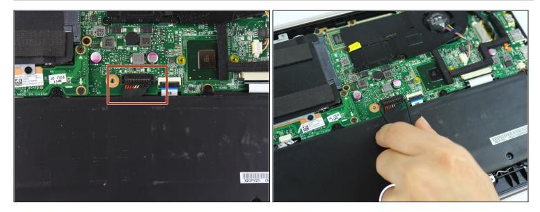
• Remove the ribbon cable with a pair of <u>tweezers</u>.
