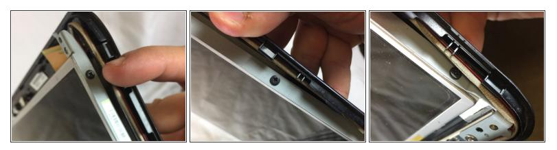
Remove the three screws on each side of the display, and place them somewhere secure.
