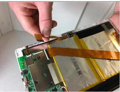
Use a plastic opening tool to flip up the ribbon cable connector that connects the camera to the motherboard.
