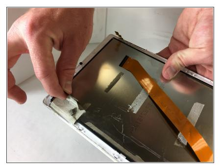
Peel away the grey mesh tape that holds down the touch digitizer's ribbon cable to the front case.
