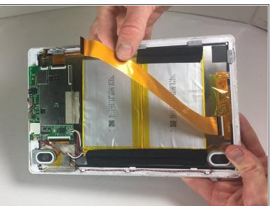
Use a plastic opening tool to flip the ribbon connector up in order to free the ribbon cable from the motherboard.
