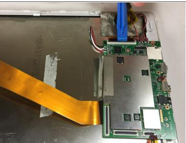
Use a plastic opening tool to flip up the ribbon cable connectors that connect the touch digitizer to the motherboard.
