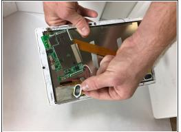
Remove the speakers from the tablet by gently pulling the yellow tape up from the front case.
