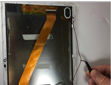
Use tweezers to free the twisted, red and black wire from the three clips on the front case.
