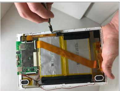
Use a Phillips head #00 screw driver to remove the thirteen screws.
