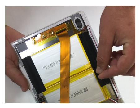
Peel the black tape up that is attached to the battery and front case.
