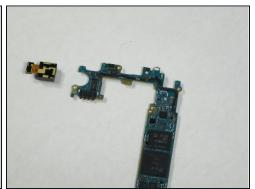
Using the plastic opening tool, remove the ribbon attaching the sensor to the motherboard.
