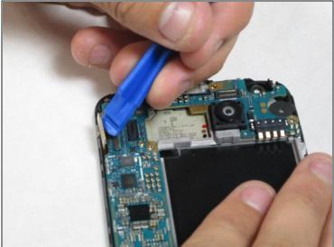
• Insert the plastic opening tool between the screen-ribbon-connector and the motherboard, then pull up. It should pop out easily.
