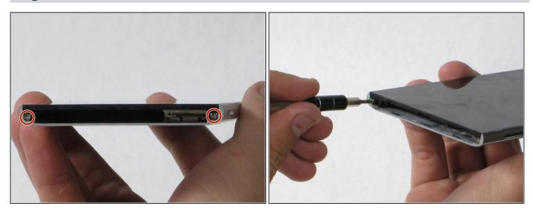
• Remove the two 5.5mm Phillips #00 screws from the base of the phone.
