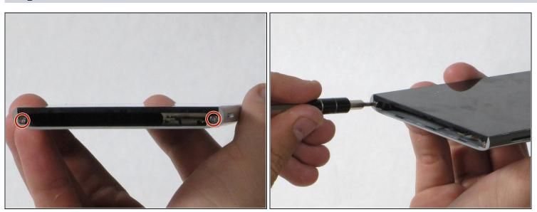
• Remove the two 5.5mm Phillips #00 screws from the base of the phone.
