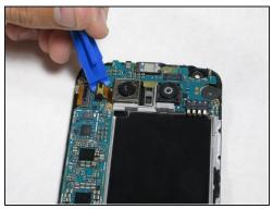
• Insert the plastic opening tool between the camera-ribbon connector and the motherboard, then pull up. It should pop out easily.
