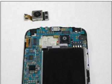
• After detaching the ribbon, carefully remove the camera using <u>tweezers</u>
