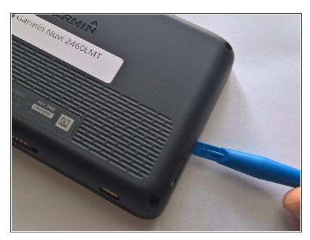
Using a plastic opening tool or similar object, find the groove in the side of the device and begin prying open the back panel. Work the tool around the entire panel until it pops off.
