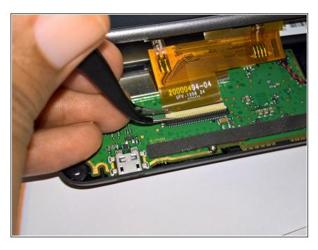
Lift the beige clamp using a tweezer or your fingernail and remove the connector.
