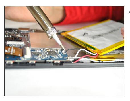
Solder the wires off that are on the battery. Use the <u>solder technique</u> <u>guide</u> for helpful tips!
