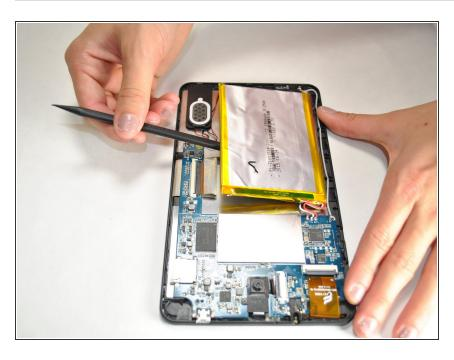
Use the nylon spudger to gently pry out the battery.
