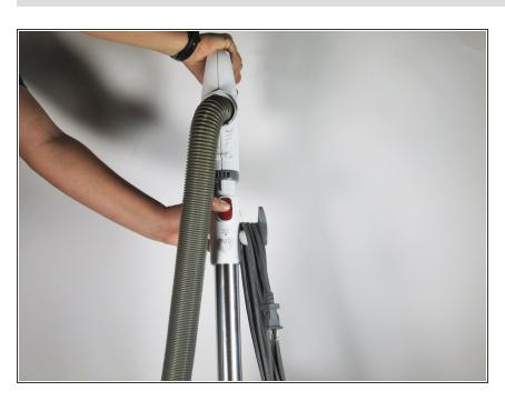
Remove the handle from the top of the vacuum with the suction hose attached.
