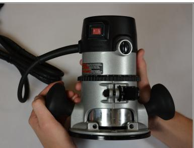
Undo the black latch located on the base of the router by pulling upwards from underneath it.
