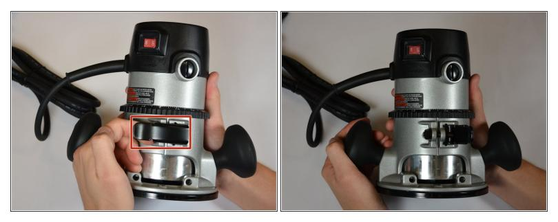
• Undo the black latch located on the base of the router by pulling upwards from underneath it.
