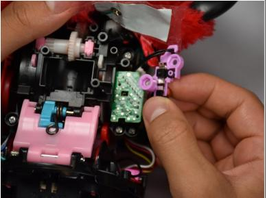
Locate and remove the two screws holding in the switch using J0 Phillips Head Screw Driver.
