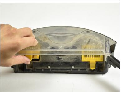
Push up on the yellow tabs on the yellow filters, and pull both filters out.
