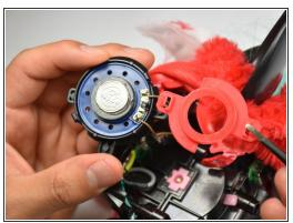
Use the blunt tweezers to pinch the latch on the speaker's casing. Detach the speaker from the both latches on both sides and remove the speaker's casing.
