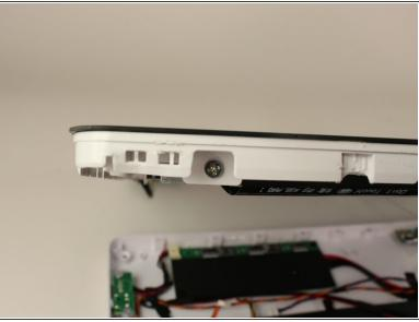
Remove each of the 6.5 mm silver screws located on the edges of the display's corners.
