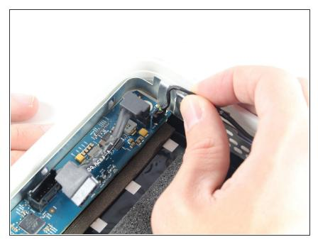
Remove the LED cable from the top left corner of the logic board by pulling the cable straight out and away from the board.
