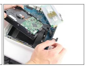
Remove the SATA connector and power connector from the end of the hard drive by simply pulling the cables straight away from the connection points.
