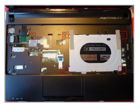
Remove the 5 screws marked with "Door".
