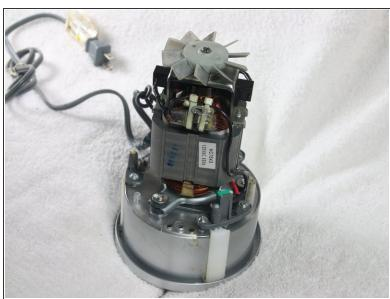
Pull off the casing from the device.
