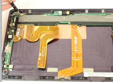
• Using a Phillips #00 screwdriver, remove six 2.5mm screws on the motherboard.
