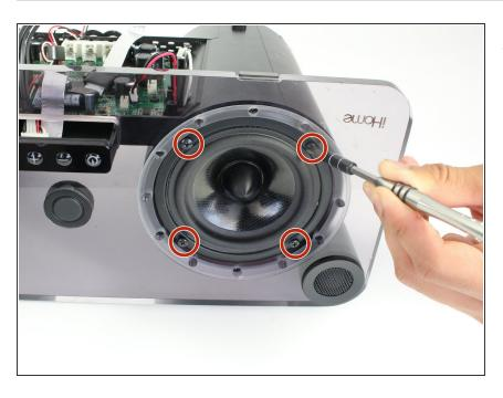
Remove the four 12.0 mm Phillips #2 screws from the edges of the speaker.
