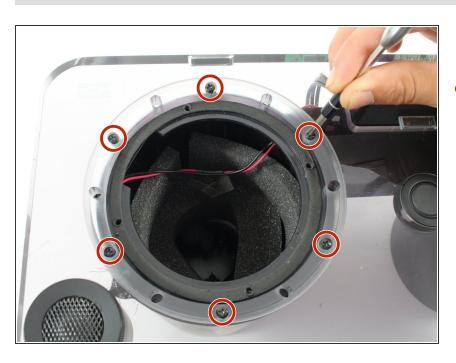
Unscrew the twelve 14.5 mm Phillips #2 screws holding the faceplate to the speaker housing. (There are six screws connecting the faceplate to each speaker.)
