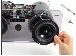
Remove the speaker from the iHome by feeding the black/white wires through the hole on the opposite side of the housing.
