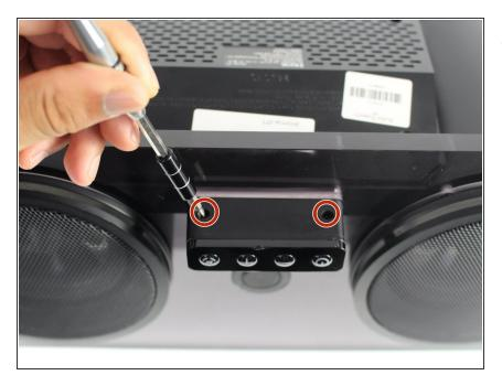
Remove the two 9.5 mm Phillips #1 screws from the dock cover.
