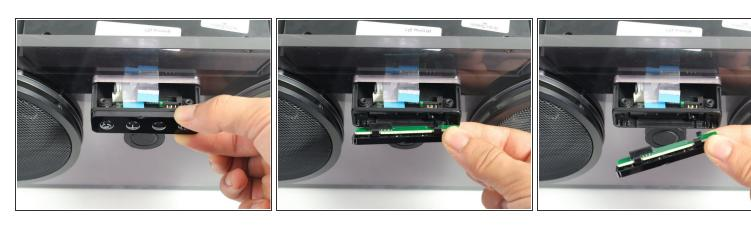
Remove the command buttons by pulling the small black panel containing them downward and away from the faceplate.
