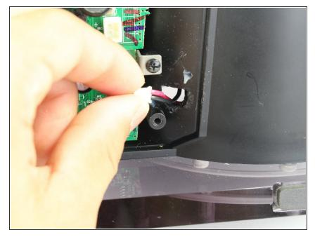
Feed the red/black wires through the hole in the speaker housing through which they stick out of. Do this to each of red/black wires you just disconnected.
