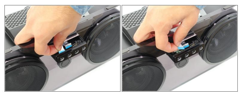
Disconnect the silver ribbon cable on the left-hand side by pulling away from the command buttons.
