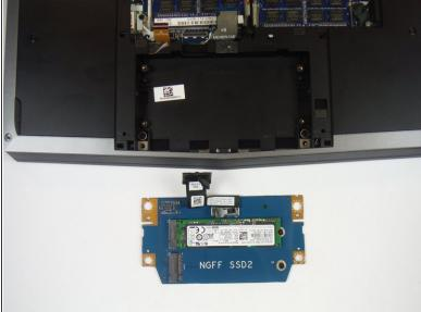
• Lift up on the solid-state drive assembly to remove it from the computer base.
