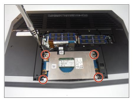
Remove (4) 6 mm Phillips head screws from the solid-state metal drive bracket, using a Phillips # 1 screwdriver.
