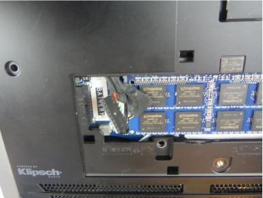
Disconnect the battery cable from the battery cable terminal.
