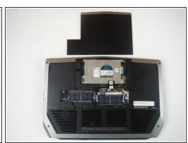
Remove the small access panel using a heavy duty spudger.
