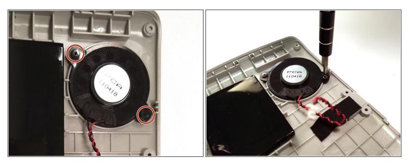
• Remove the two 4mm Phillips #00 screws securing the speaker assembly and remove speaker.
