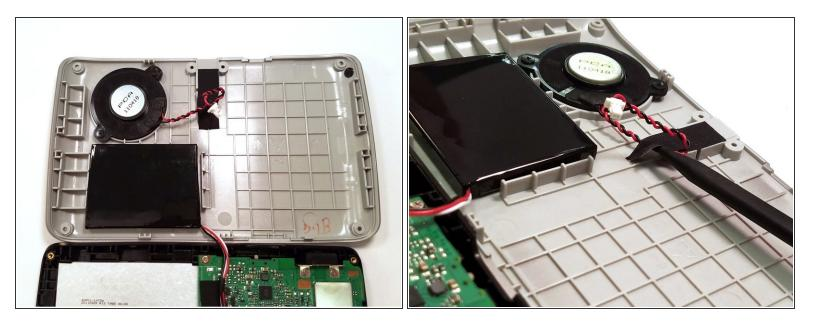
• Open the device and remove the tape from the speaker wire using the spudger.
