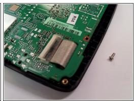
There will be two 5mm Phillips #00 screws that need to be removed from the motherboard.
