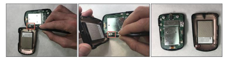
• Use the blunt <u>tweezers</u> to unplug the battery cable from the PCB board. Grab the battery cable plug from the sides.
