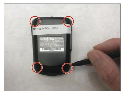
Remove the rubber screw caps using the pointed tip of the Spudger.
