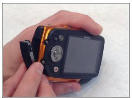
To begin, open the the battery hatch on the right side of the camera, relative to the LCD screen. The battery hatch is the larger of the two. To open, simply slide the black button in the direction of the arrow next to it and the hatch will pop open.
