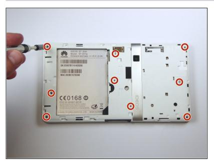
With a T5 hexagonal head, remove the nine black 2.5 mm torx screws. Place them carefully aside on the magnetic mat.
