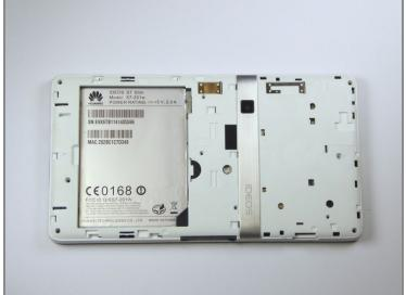
• Using a plastic opening tool, pry off the top cover casing gently by moving the tool along all three sides.
