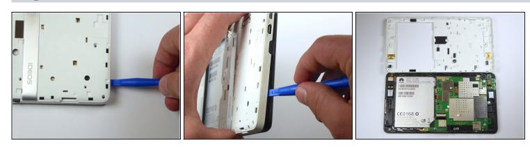
• Using a plastic opening tool, pry off the back casing gently on each side of the tablet.
