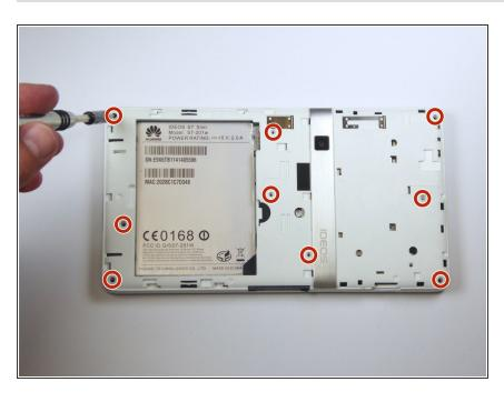
With a T5 hexagonal head, remove the nine black 2.5 mm torx screws.
