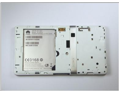
Using a plastic opening tool, pry off the top cover casing gently by moving the tool along all three sides.
