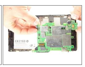
Disconnect the five cables connected to the logic board and then carefully lift the logic board out of the casing.
