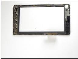
Tilt the tablet on its lengthy side, place your thumbs on the side and gently separate the LCD from the touchscreen.
