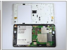
Using a plastic opening tool, pry off the back casing gently on each side of the tablet.
