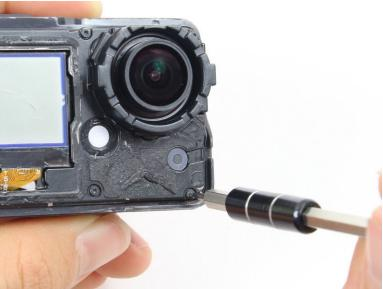
Remove the six T3 Torx screws.
