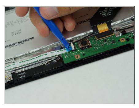
Using a plastic opening tool, lift the white tab holding the power button cable, located on the camera board and pull out the cable strip.
