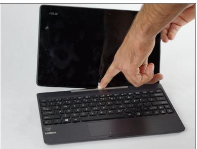
Detach and separate the screen from the keyboard by pressing the silver release button at the base of the tablet.
