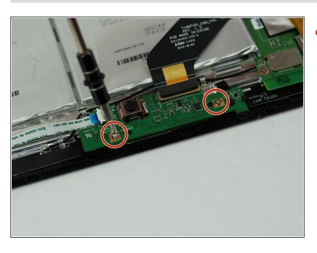
Unscrew two 5mm screws from the camera board using a Phillips #0 Screwdriver.
