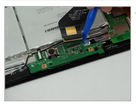
Also using the plastic opening tool, gently lift up and remove the large black strip connecting the camera board to the motherboard.
