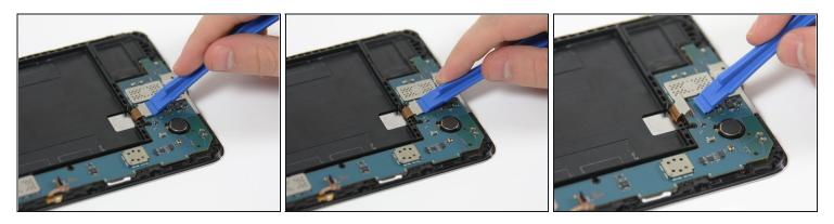
• Disconnect the wire near the bottom of the motherboard by placing the plastic opening tool under the edge of the connector to flip it up.
