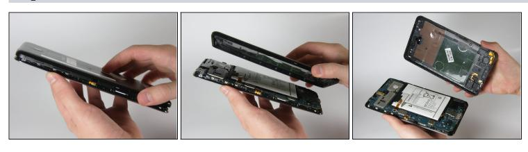
• Carefully remove the back panel from the frame of the device.
