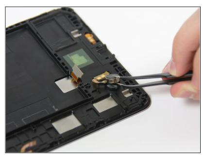
• Using the <u>tweezers</u>, pull the vibrator off the board.
