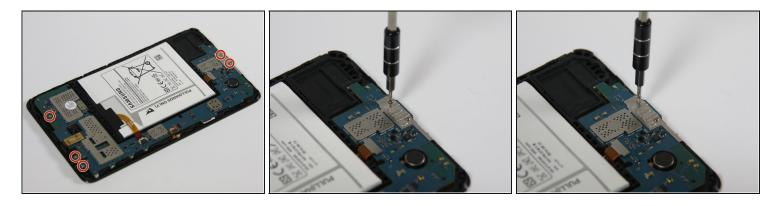
• Using a Phillips #00 Screwdriver, remove the five 4 mm screws connecting the motherboard to the frame of the device.
