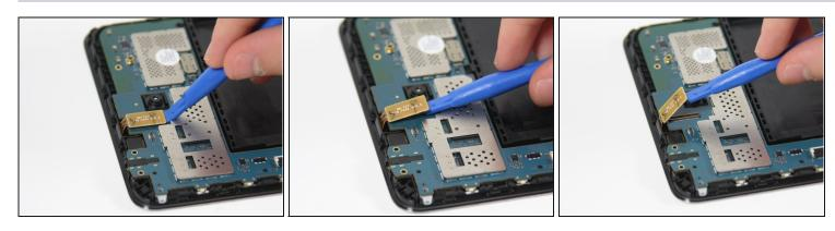
• Disconnect the wire near the top of the motherboard by placing the plastic opening tool under the edge of the connector to flip it up.
