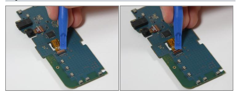
• Use a plastic opening tool to unlock the rear-facing camera wire from the motherboard by flipping up the retaining flap.
