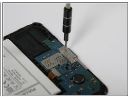
Using a Phillips #00 Screwdriver, remove the five 4 mm screws connecting the motherboard to the frame of the device.
