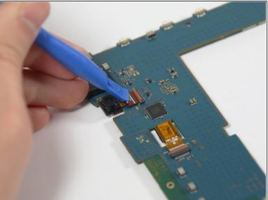
Use a plastic opening tool to unlock the front-facing camera wire from the motherboard by flippingup the retainer flap.
