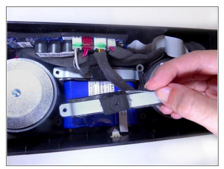
• Remove the two brackets that hold down the battery using your hands.
