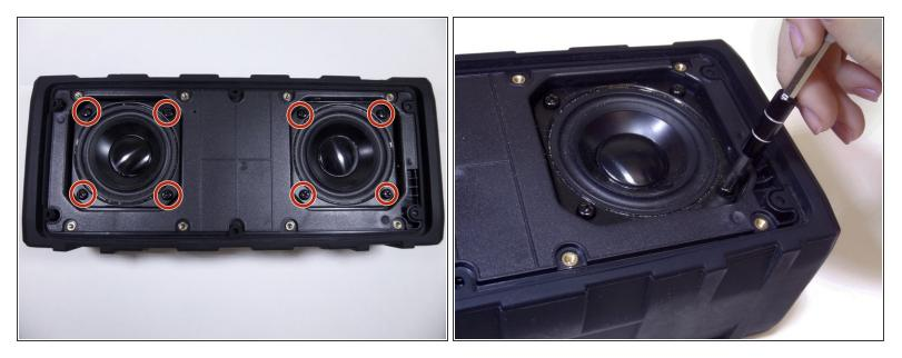
Position the device facing up and remove eight 10mm Phillips head screws using a J1 Phillips head screwdriver.
