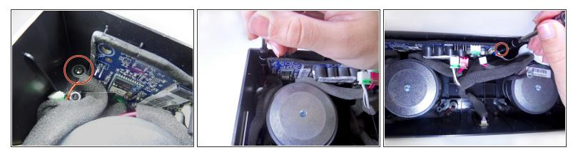
Locating the two screws on either side of the motherboard, unscrew the two 8 mm Phillips head screws using a J1 Phillips head screw driver.
