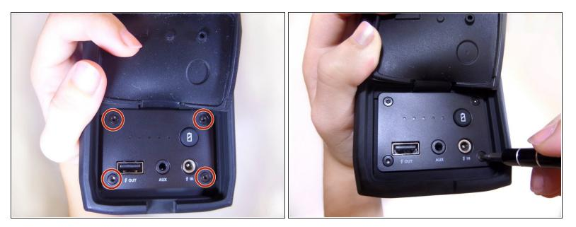
Turning the device on its side, unscrew the four 15mm hexagon 2.0 screws on the charging port panel.
